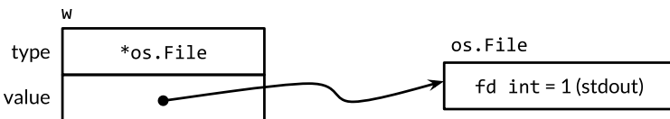
Figure 7.2. An interface value containing an *os.File pointer.
