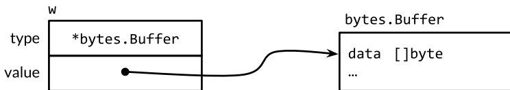
Figure 7.3. An interface value containing a *bytes.Buffer pointer.
