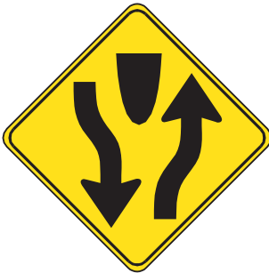
Two-lane highway ends; divided highway begins.
