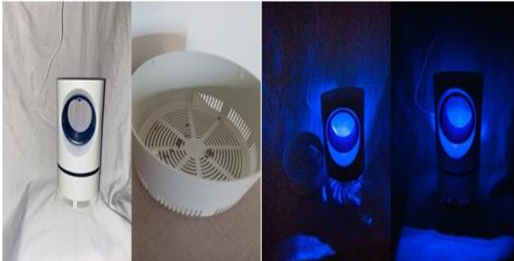
Figure (1): Ultraviolet light trap with a fan.
