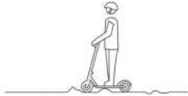
⚠ Do not ride quickly over uneven surfaces. Keep a speed between 5km/h and 10km/h and bend your knees slightly to ensure maximum safety.
