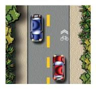
**Bicycle lanes** are indicated by a solid or dashed white line or green pavement markings, and a bicyclist symbol. A bicycle lane is for the preferential use of bicyclists. Drivers should not drive in the bicycle lane except when necessary to turn left or right. Before turning, check your mirrors for bicyclists that may be behind you and yield to bicycles in the lane.
