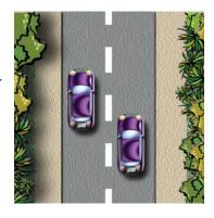
**Dotted white lines** are actually small rectangles in a series where each is closely spaced to the next. They are used to show lane assignment in intersections and interchanges where there might otherwise be a tendency to drift out of a lane or an area of intended use. Often they are used to guide two turning lanes through the intersection. Dotted white lines are also used to denote the opening of a turn lane at an intersection and entrance/exit lanes at interchanges.
