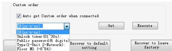
While using as **Unit card reader**, choose “ID(xx-xx-xx):” and input the Building No., Unit No. and Device No. behind it. For example: to set as building No.1, unit No.2 and device No.3,
