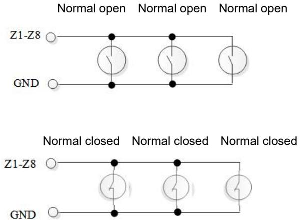
**NOTE: Unused defense area interfaces could be closed in the Alarm System Setting, or it can be blocked by 10K resistance.**
