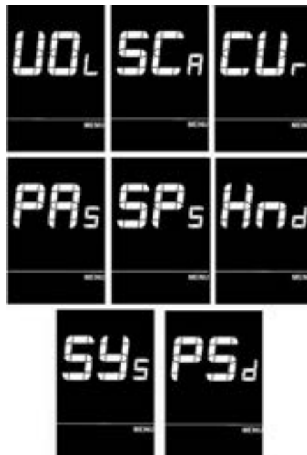
Personalized parameter setting interface
