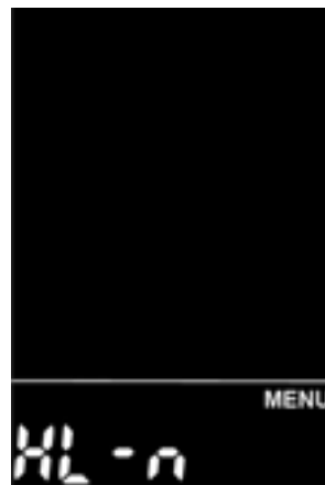
Throttle assist push setting interface
