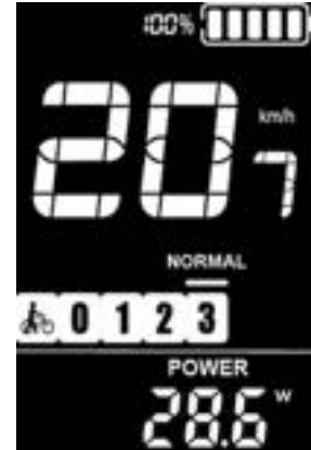
Motor Power Indication interface
