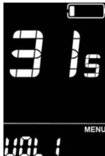
Battery level setting interface
