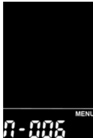
PAS disk magnet number setting interface
