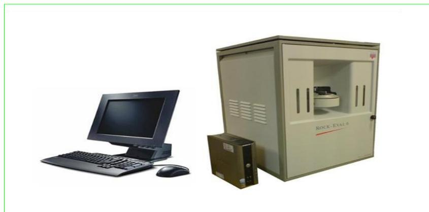
**Fig. 2. Illustrative picture showing the Rock-Eval 6 apparatus**
