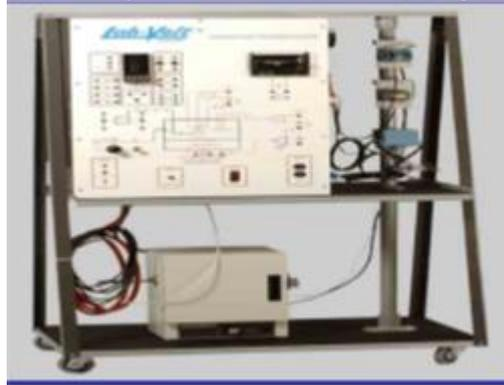
Figure 2: Lab-volt temperature process
