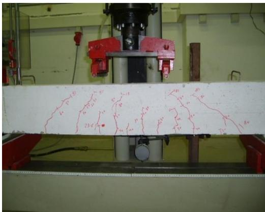
Figure (15) Failure for sample B1
