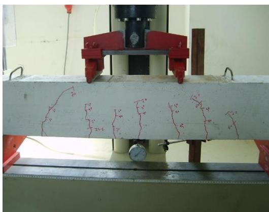
Figure (23) Failure for sample B10
