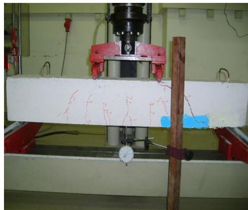
Figure (16) Failure for sample B2
