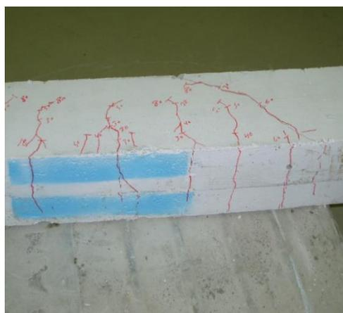
Figure (24) Failure for sample B11
