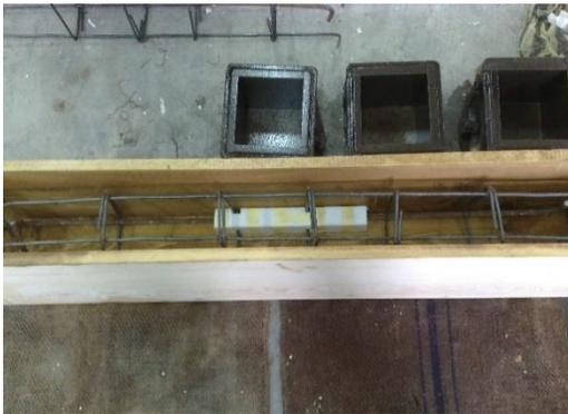
Figure (2) shape of the mould ready to cast
