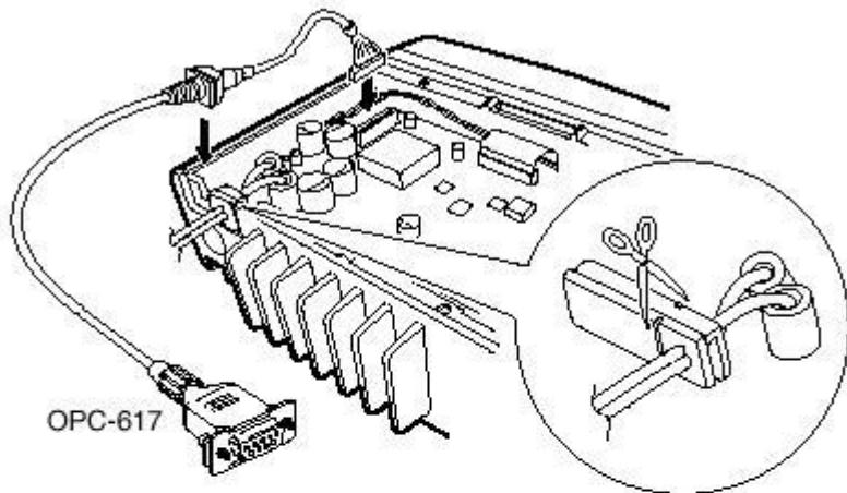
Cut off the bushing as in the illustration, when you install the optional OPC-617.
