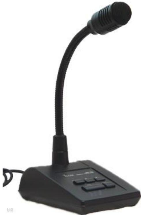
The **Icom SM-50** is a unidirectional, dynamic microphone designed for base station operation with select Icom transceivers. (It cannot be used with non-Icom transceivers since the power is supplied from the connected transceiver). The SM-50 features Up-Down tuning (on compatible ICOM transceivers). There is a switch for PTT (push to talk) and also a lock feature. There is also a Low Cut Switch on the top of the base to cut out the low frequency components on input voice signals.
