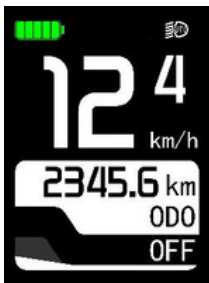
Sufficient battery level
